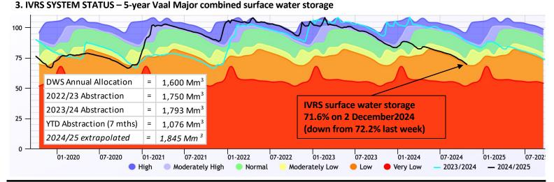
The 5-year Vaal Major system storage is shown as an indication that it is tracking lower than in the previous 3 years. DWS Restrictions are implemented on the IVRS when dam levels are below 60% at the beginning of the hydrological year starting in May of each year. Should over-abstraction continue, and rainfall be lower than normal, the DWS model is likely to indicate that restrictions be imposed in May 2025. Sources:
